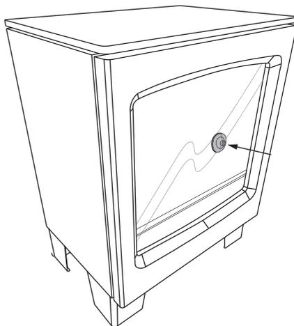
2. Lift the glass up and carefully slide out of the fire.
