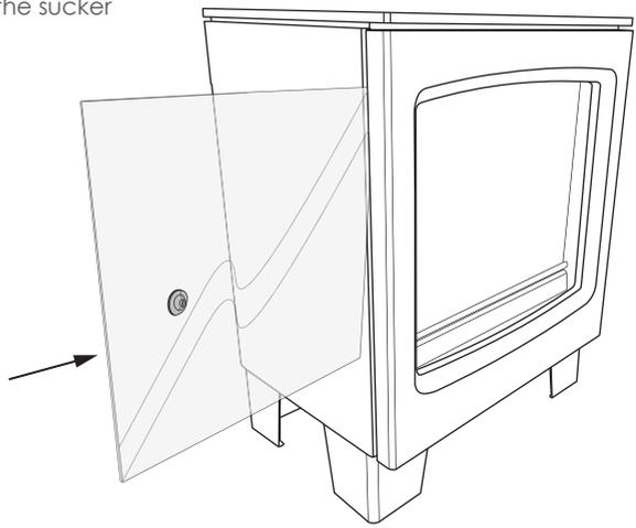
2. When inserted over half way, move the sucker pad to the glass inside the fire.
