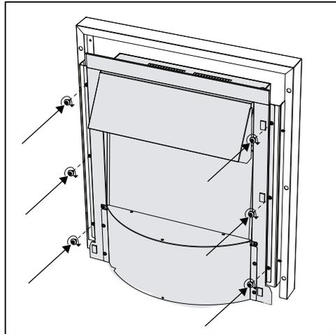
Attach inset fire to spacer, using self tapping screws provided, & screw driver.
