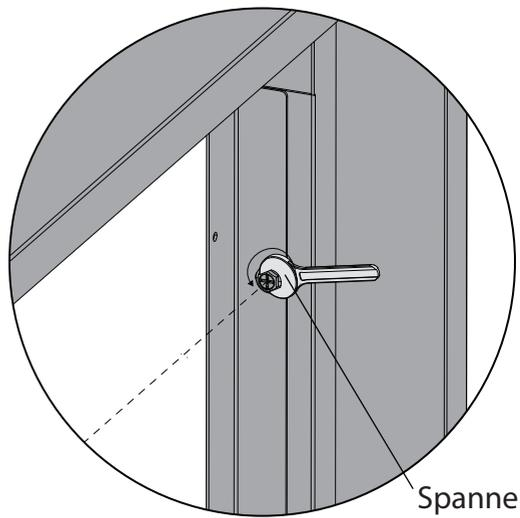
Ensure two brackets are fastened loosely, not tight. If tight, loosen with spanner provided.
