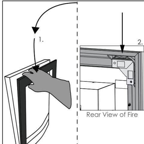
Position the bottom of the trim behind the locating brackets on the fire, push the trim forward at the top, and then drop down, ensuring the fire locates within the corners of the trim. Then push down.
