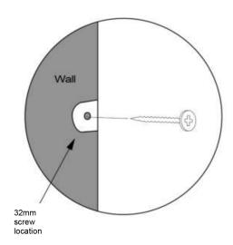
**Note** if fitting the cover to plaster board with a cavity behind then propriety wall fixings (not supplied) will be required.
