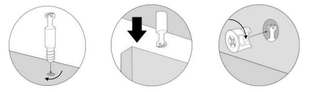
Using a screwdriver and cam dowels, assemble the legs, top and fascia as shown
