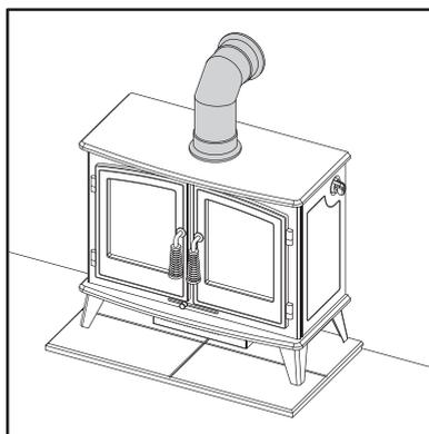
4. To position the split batten, measure a MINIMUM distance of 75mm from the top of the stove pipe to the bottom of the split batten and mark the wall.
